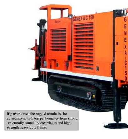
Hydraulic leveling jacks make set-up fast and easy and stabilize the rig to an ideal drilling position
