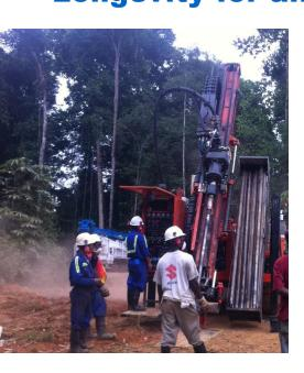
AC/150 has solid engine that coupled with onboard air compressor by clutch, provide perfect combination for any drilling condition. Additional factors like load sensing and fan speed controls add performance
